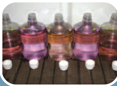
> Sample processing: Potassium permanganate is added to sea water samples as a first step towards isolating actinium. (Photo: C. Hanfland)
