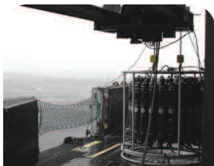
> A CTD with 24 bottles is ready for deployment to sample ^{227}\text{Ac} in the Weddell Gyre. Due to the minute concentrations of actinium, about 50 L of sea water are required for a single analysis.
